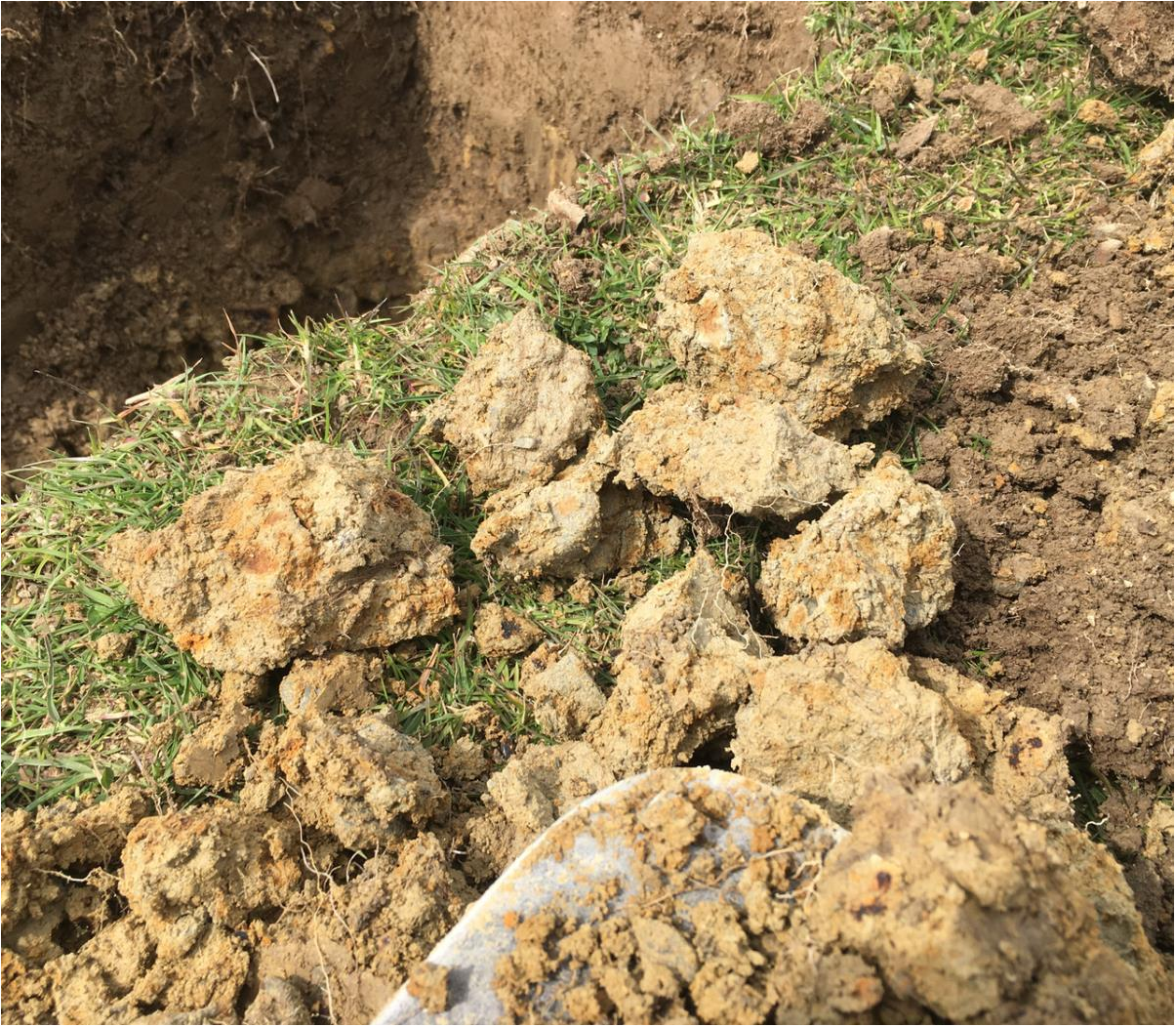
Photo 1 of Subsoil in pit at AB14, Site C. Moderately developed, Coarse SAB, friable. NOT SPL.
