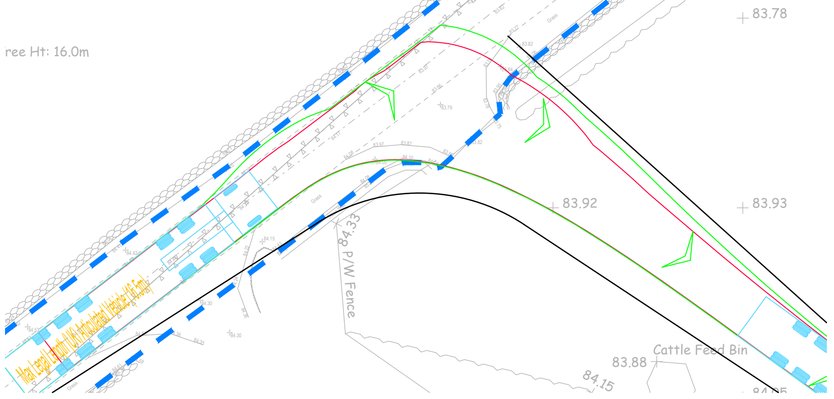
Articulated HGV Turning Right Into Access Scale 1:200
